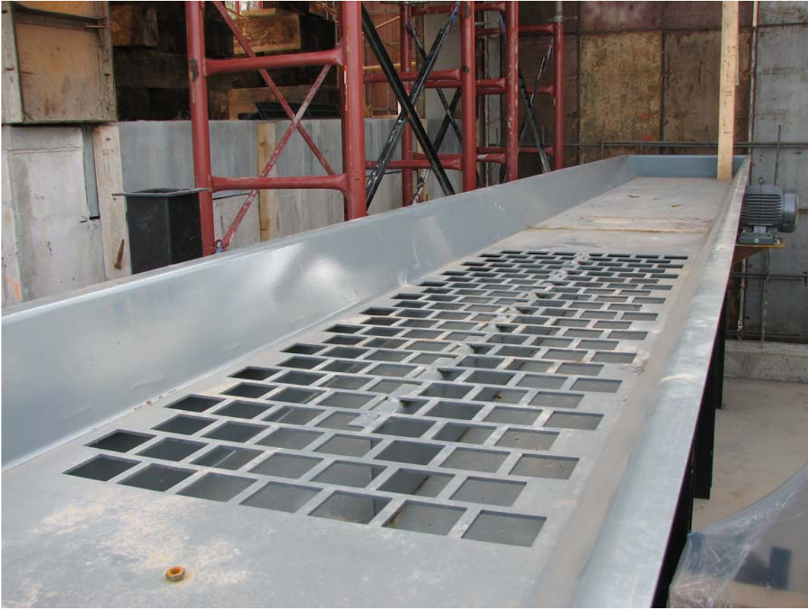
Vibratory fuel conveyor and screen -- not in final position (approx. 2-in. square screen – eyeball estimate)
